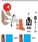
Fast stroke SH starting at EJ150-3S with 3-times the speed of the regular stroke NH.
