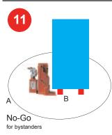
Always make sure that bystanders and children are away from the work area. Cordon off a No-Go area with cones or tape etc. The NO-GO area must be the area of the load plus a radius around the load of at least 1,5 times the highest dimension of the load. This is the operators responsibility (A) Make sure that the load is supported during the lifting and lowering process (B). Under load the jack should never be left unattended and should stay in the same position for only a short period of time.
